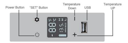
• Power On/Off: Press the Power Button (1) to turn the unit on/off
